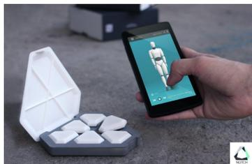
A company called Notch, of New York, is producing a 3D motion sensor pack that tracks total body movement via six triangular sensors that can be placed anywhere on the body. Each sensor comprises an accelerometer, gyroscope and compass, and physiotherapists use the data captured to help improve patients' range of motion. Notch has just shipped its first wave of devices and is accepting orders for more, for delivery very soon. It is already used in universities, labs and companies worldwide.
